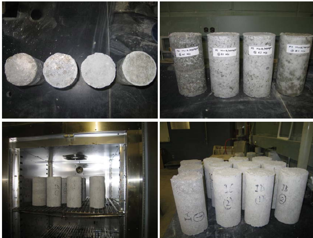
Figure 26 Oven drying of cylinders for moisture content determination
