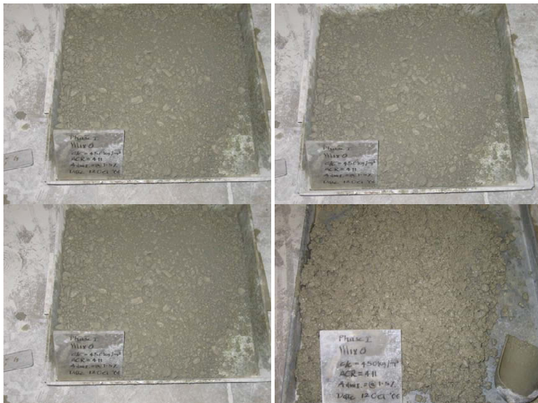
Figure 25 Mixes at different moisture contents
