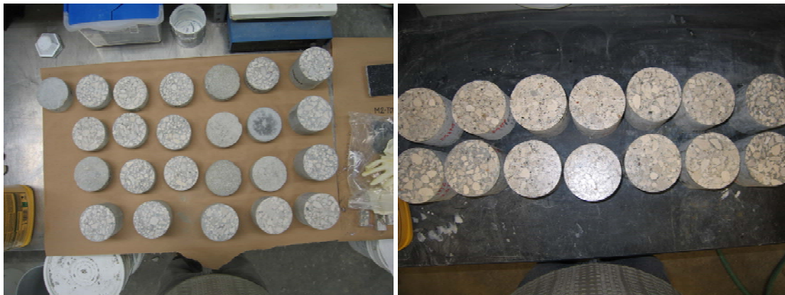
Figure 29 Sample coating for sorptivity samples
