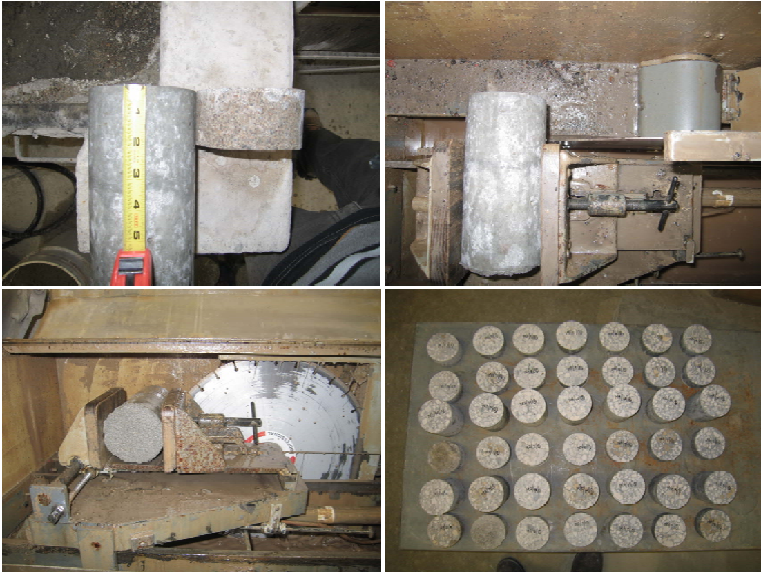
Figure 33 Cutting of slices for voids content
