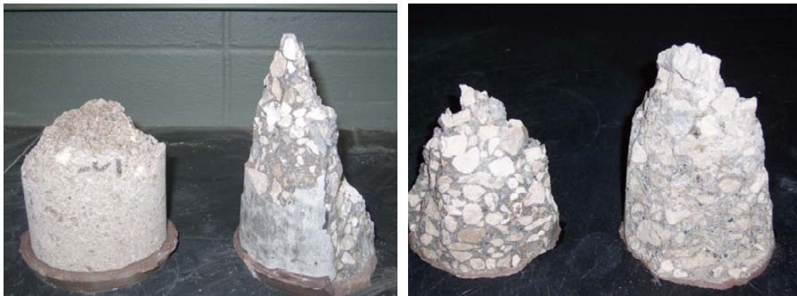
Figure 41 Cracking pattern in compressive strength test cylinders
